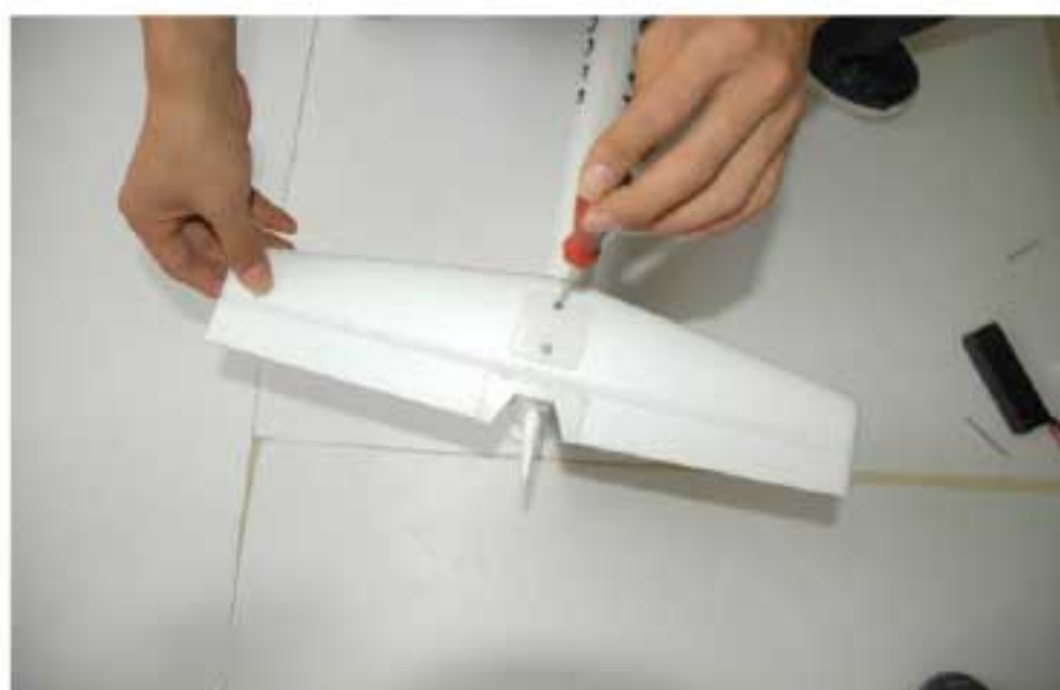
9. Install the elevator. Screw-PA3.5*20(2PCS)
