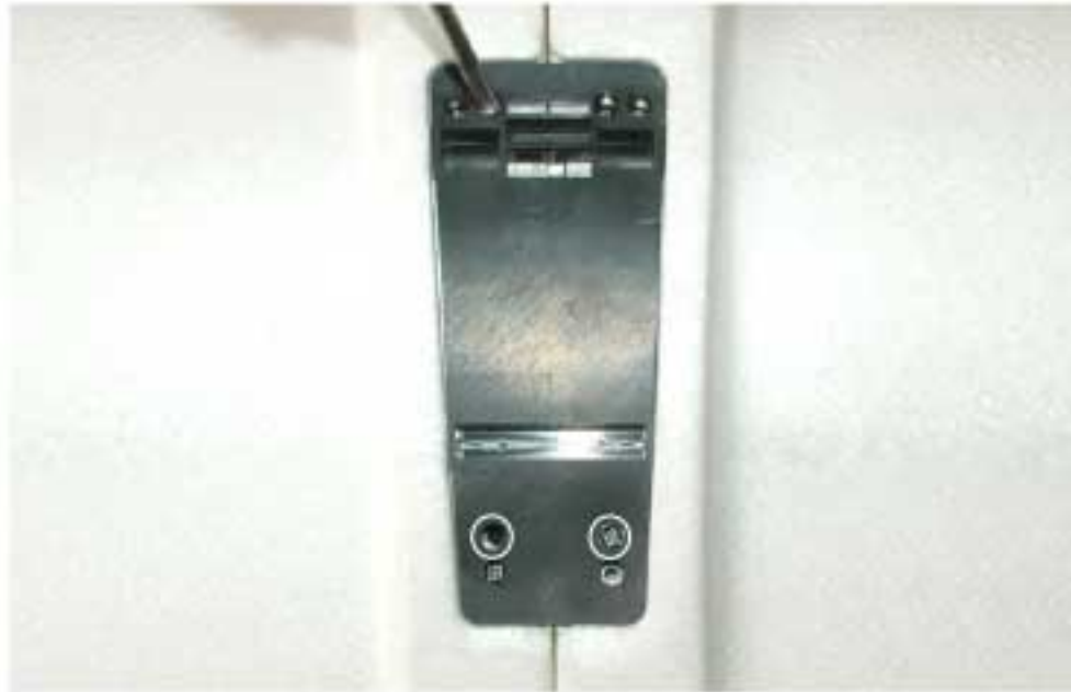
6. Secure the main wing. Screw-PM3.0*50(4PCS)
