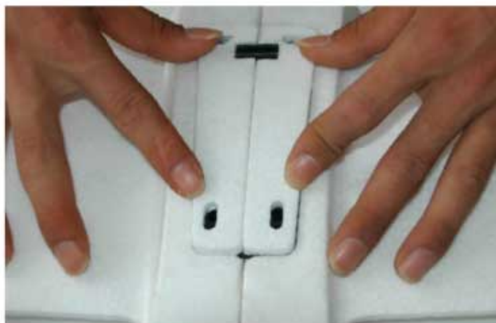
6. Secure the main wing. Screw-PM3.0*50(4PCS)
